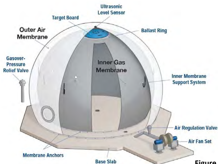
Figure 5-6 Typical Gas Membrane Storage System Figure Courtesy of WesTech
