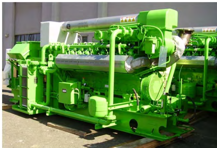
Figure 5-3 GE Jenbacher 850 kW IC Engine
