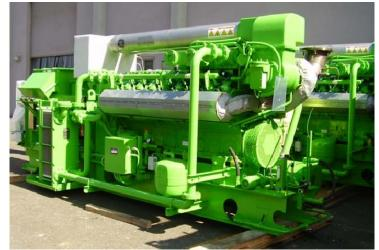
Figure 3-4 GE Jenbacher 850 kW IC Engine
